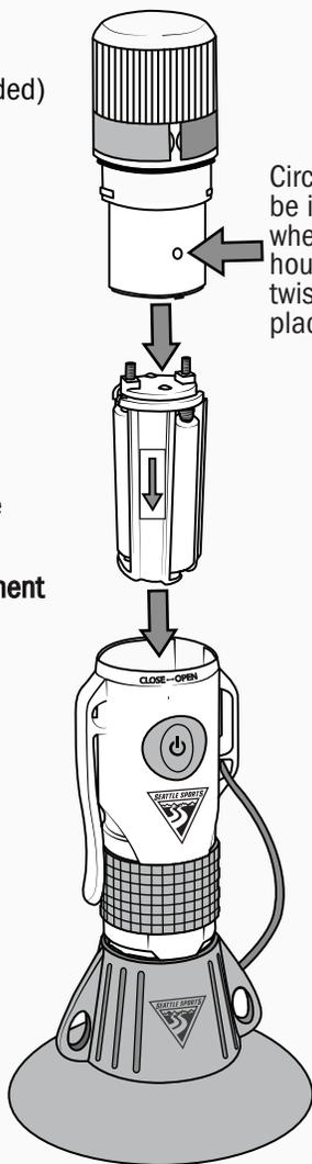
Circle should be in front when light housing is twisted into place
